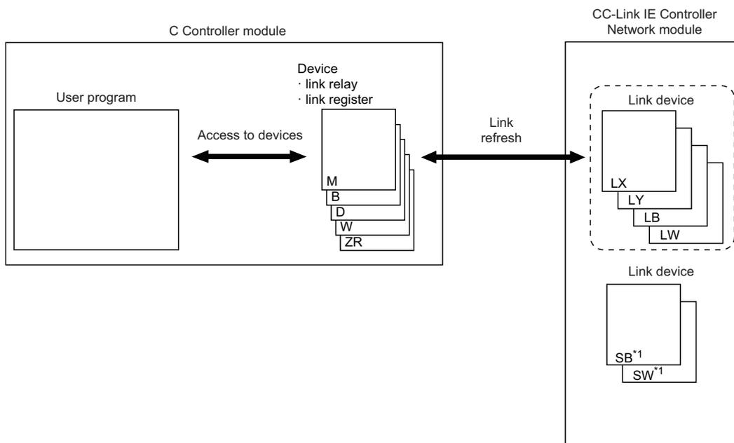
\*1 Link refresh cannot be performed for SB/SW. Use the direct access.
