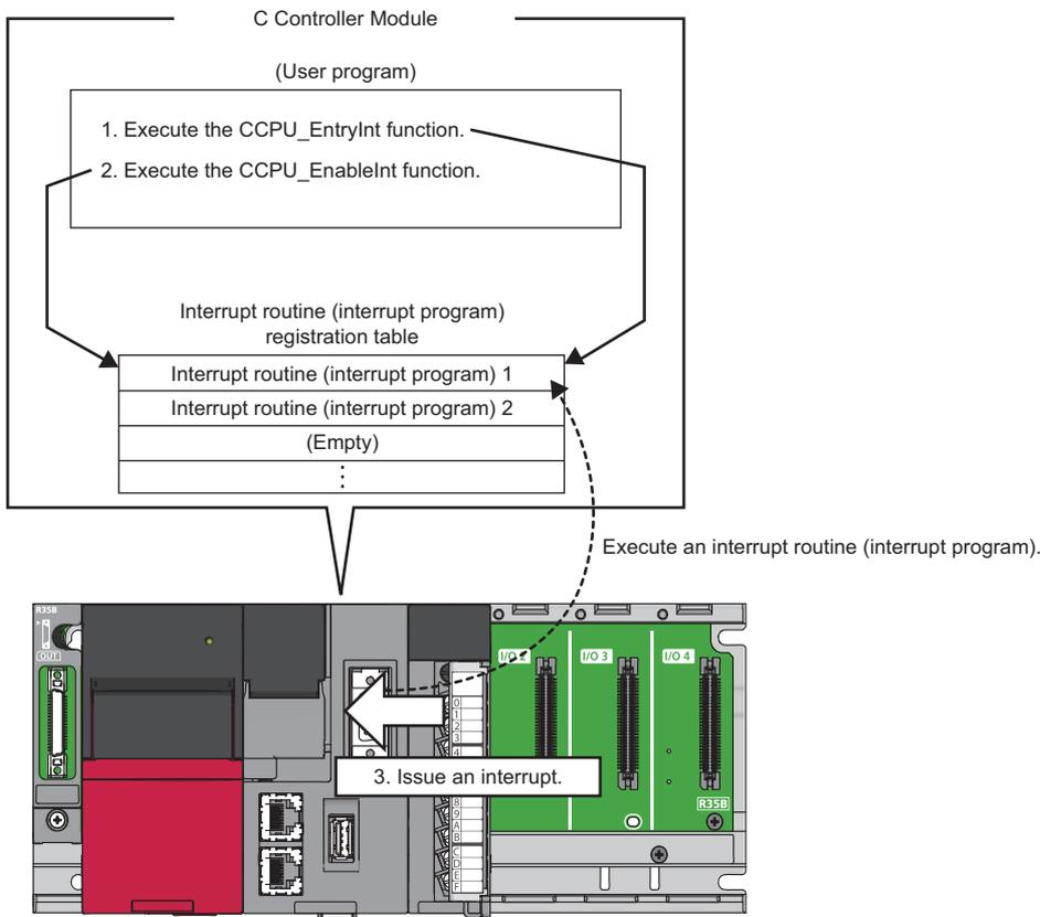
1. By using the C Controller module dedicated function (CCPU\_EntryInt), register a routine (user program) to be called as an interrupt routine (interrupt program) when an interrupt is requested.
