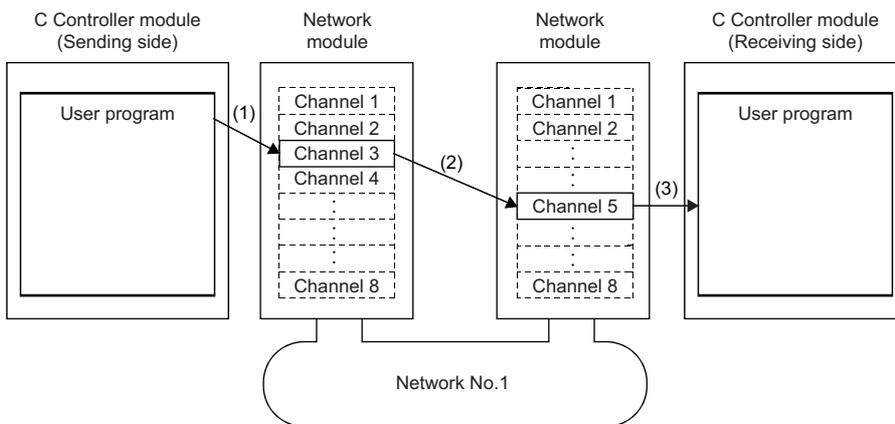
(1): The sending side C Controller module sends data by specifying the channel used in the own station and the channel used in the target station with the message send function of a user program.
