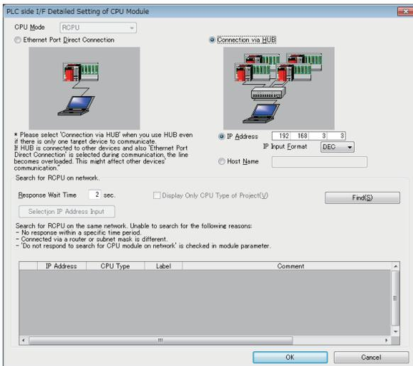
4. Set the module to be connected to "PLC side I/F".
