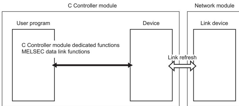
The following shows the functions used to access devices by link refresh.
