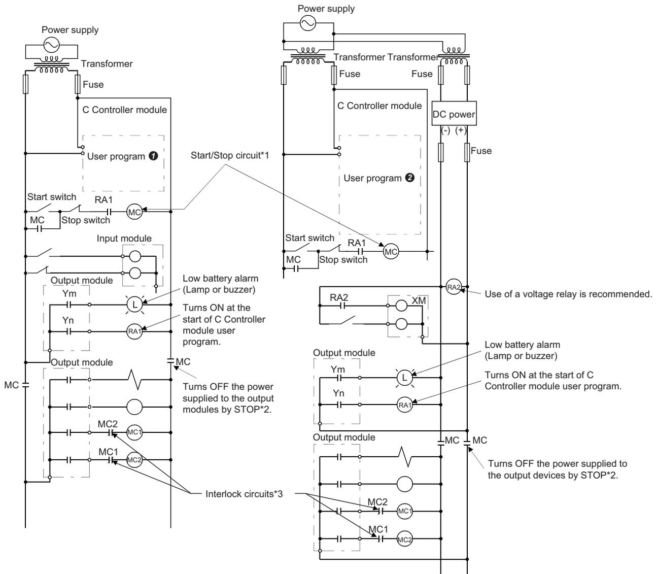
\*1 The C Controller module starts when RA1 (control starting output) turns ON.
