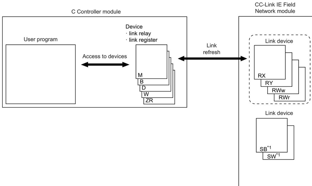
\*1 Link refresh cannot be performed for SB/SW. Use the direct access or buffer memory access.
