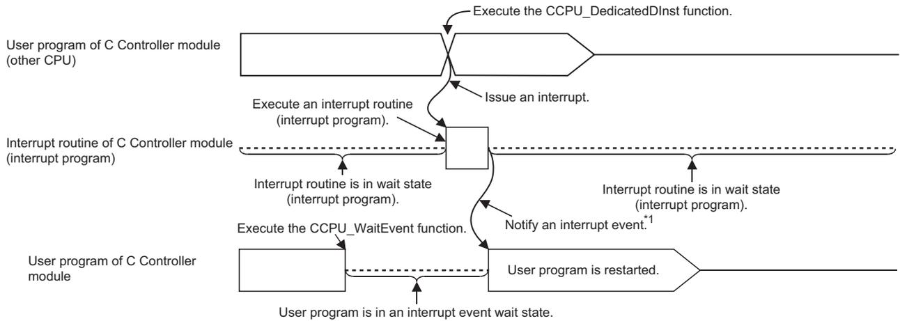
\*1: The interrupt event is notified after the interrupt routine (interrupt program) is completed.
