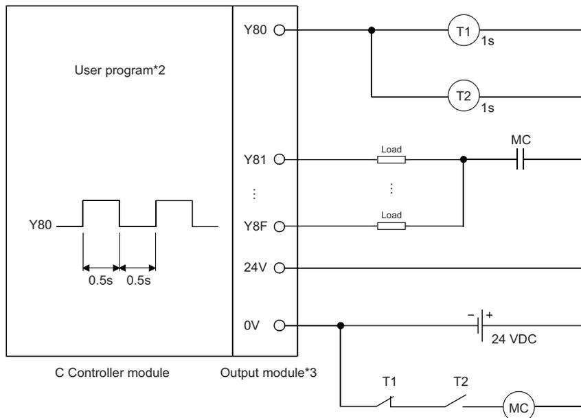
\*2 Create a program to make Y80 repeats ON and OFF at the interval of 0.5 seconds.
