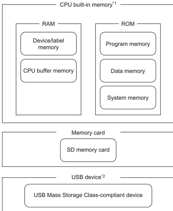
\*1 CPU built-in memory is a generic term for the built-in memory in a C Controller module.
