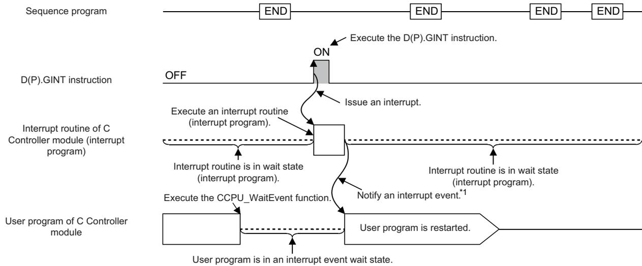
\*1: The interrupt event is notified after the interrupt routine (interrupt program) is completed.
