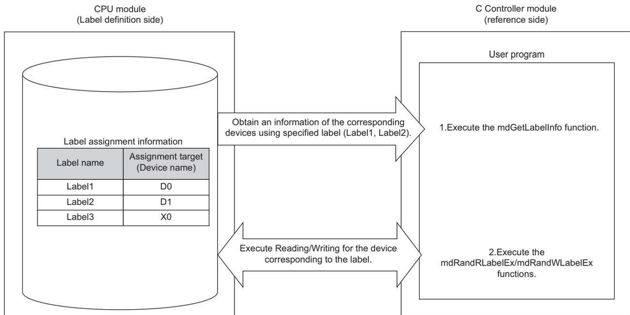
1. Acquire label assignment information (device information) of the specified label by using the MELSEC data link function (mdGetLabelInfo).
