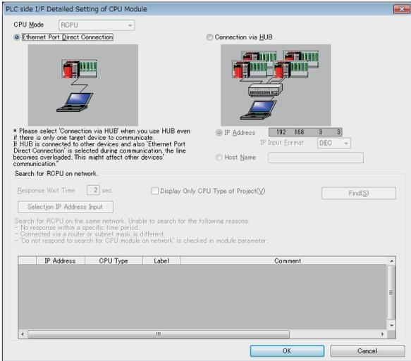
4. Set the module to be connected to "PLC side I/F".
