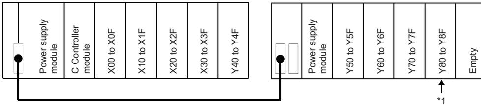
\*1 Mount an output module for fail-safe purpose on the last slot of the system. (In the example above, the output module is mounted on Y80 to Y8F.)
