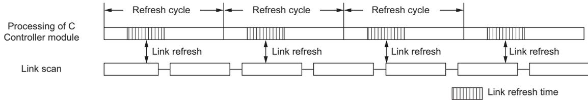
When the station-based block data assurance is set, cyclic data consistency is assured in station units since the C Controller module does refresh cycle with a network module by handshaking.
